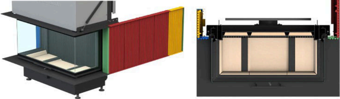
... detail (schematic) "Start-left" (blue), "Start-right" (green), "1-piece" (yellow) and "2-piece" (red) modules
